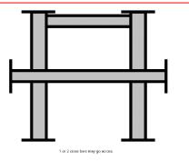
These two diagrams are a guideline to how the frame should be constructed but gusseting or triangulation is accepted.
